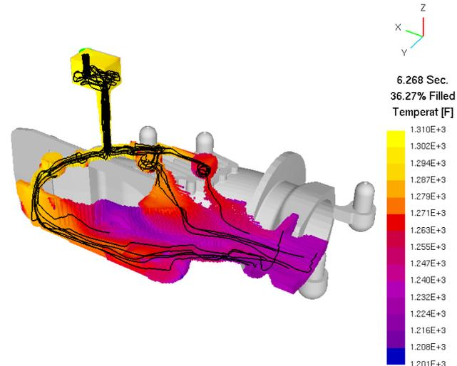
**Flow Path Tracing in an Aluminum Sand Casting**
