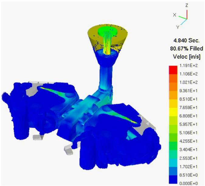
**Metal Velocity Prior to Misrun in two Copper Sand Castings**
