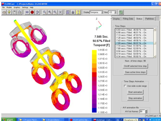
Initial Filling of Aluminum Castings Showing Metal Temperature in the Tilting Die. Permanent Mold Process.
