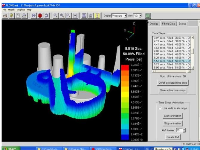
Metal Velocity Plot During the Filling Sequence. Aluminum Permanent Mold Process.
