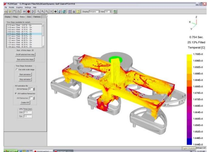
Initial Filling of Steel Castings Showing Metal Temperature. Investment Casting Process.
