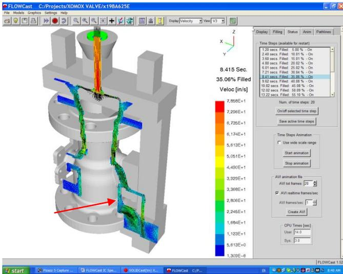
**Velocity Vectors Show Reverse Flow OUT of the Casting and INTO the Gating System. Investment Cast Valve Body.**
